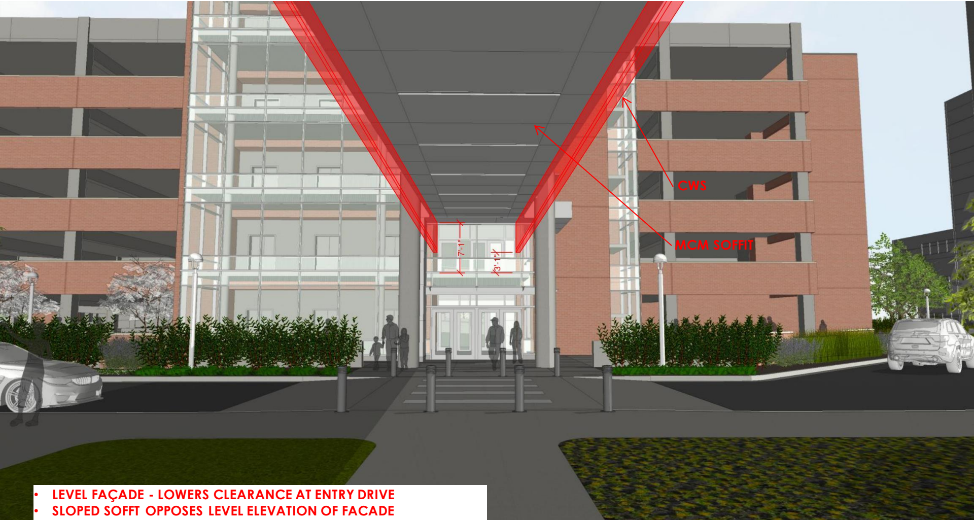
Sloped Soffit With Level Curtain Wall
