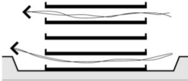
OPEN PARKING STRUCTURE WITH NATURAL VENTILATION
